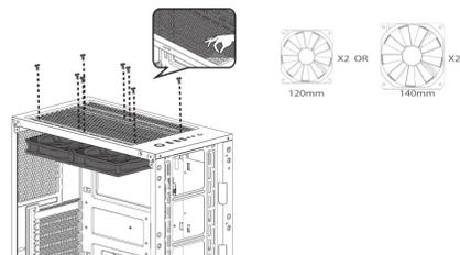
**8 Front/Rear Fan Installation/ /Installation du ventilateur**
