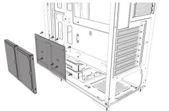
**6 3.5" HDD Installation and 2.5"SSD Installation(2)**
